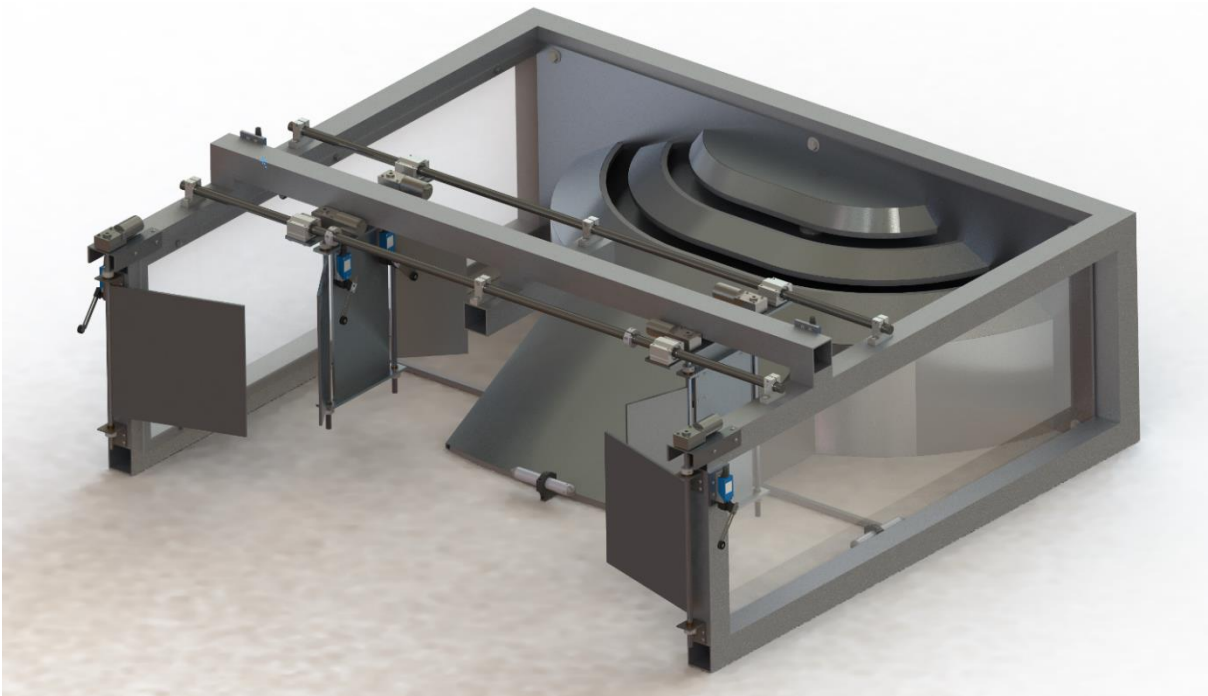
Figure 1: Overtopping Test Rig – Isometric View
